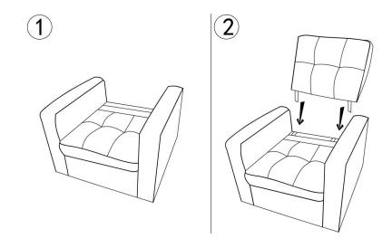
2) Put the back part slide into the seat.
