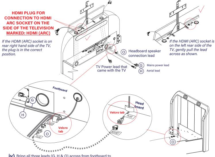
iv) Bring all three leads (G, H & O) across from footboard to headboard in a straight line, fix to velcro tab at each end.
