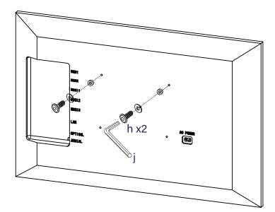
ii) When spacers are provided it is very important that these are fitted in the correct place, fit between television & the TV mounting bracket (x) as in this sketch. The spacers are needed to keep the TV screen vertical.
