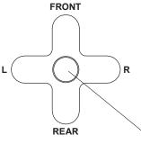
Press the button marked Front and the sound level will be higher at the footend than the headend of the bed.
