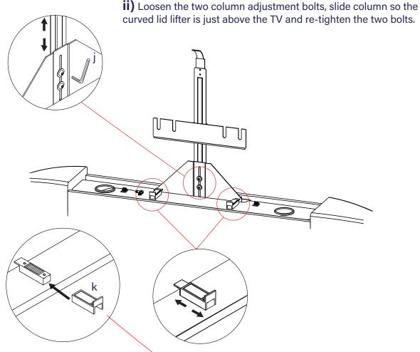
**iii)** The upper part of each support (k) slides to hold front of television in place, please follow the instructions on how to correctly set these supports in Step 9.
