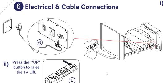
plug the small power plug on one end of the mains power lead (G) into the socket at the bottom of the footboard. On the other end of the lead, bring the 3 pin plug out under the headboard and connect it to your wall socket - for safety this must be an earthed power supply.
