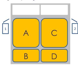
There are 4 heating zones operated by two controllers. In the image, areas "A" and "B" are controlled via controller "1". Areas "C" and "D" are controlled via controller "2".
