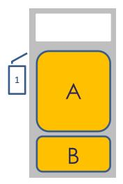
There are 2 heating zones operated by one controller. In the image, area "A"'s temperature relates to the upper body heat setting that is selected using the "Body" button on the controller.
