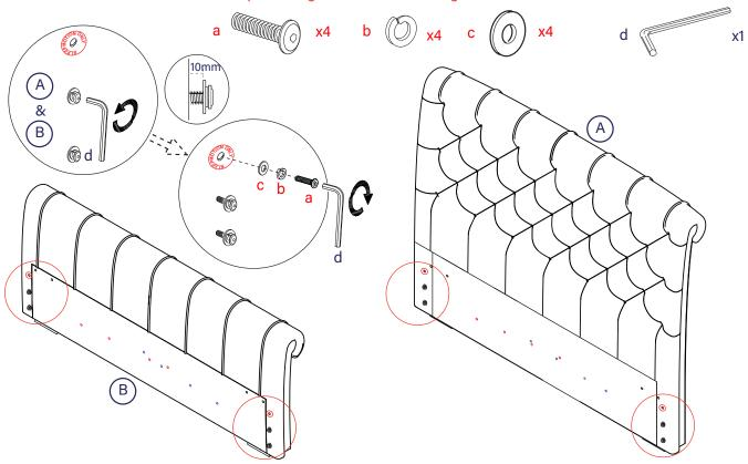
To the prepared headboard, fit the right hand side rail.
