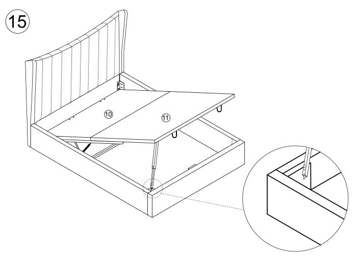
Fix the metal tube to the slot as in the picture.
