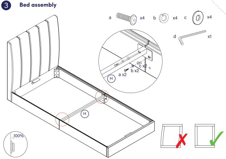
Make certain the bed is squared up as shown in the diagram then tighten all bed assembly bolts 100%.
