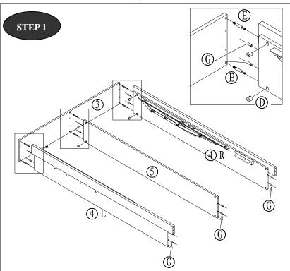
1) Assemble footboard panels (2&3) to the side rails (4R&4L). Secure by tightening the locking nuts in the same way as described in step 1.
