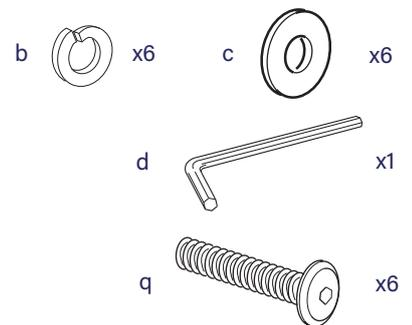
ii) Using Hardware Pack (A), unfold and bolt each wing to the main headboard. Screw three bolt sets (q, b & c) into the pre-tapped holes on each side, tighten with allen key (d).
