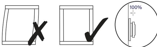
**8** Check that there is the correct gap around the perimeter of the bed base
