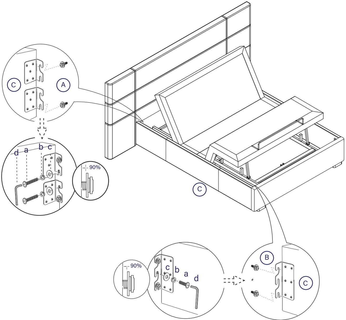
Make certain the bed is squared up as shown in the diagram then tighten all bed assembly bolts 100%.
