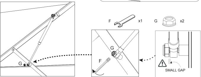
Hold up each arm and slide piston stem onto the threaded axle and fit nut (G) using spanner (F).
