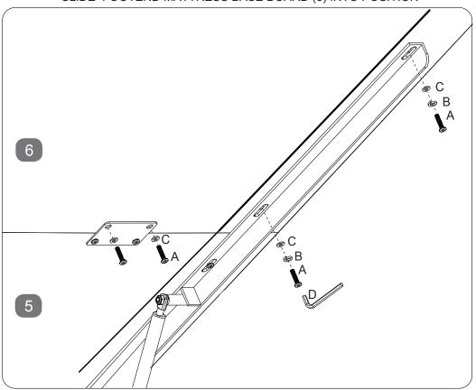
LOOSLEY CONNECT THE PLATES SCREWING ALL 8 SETS OF BOLTS INTO PLACE
