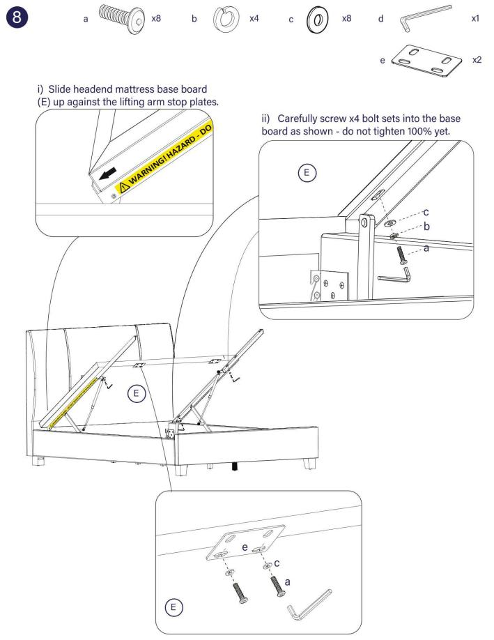
iii) Fit both connection plates (e) to headboard mattress base board (E) as shown, (before fitting second mattress base F).
