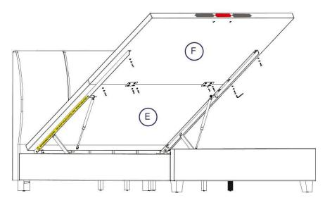
ii) Loosely connect plates (c) to (F) then screw other x4 bolt sets through the supports into the base board.
