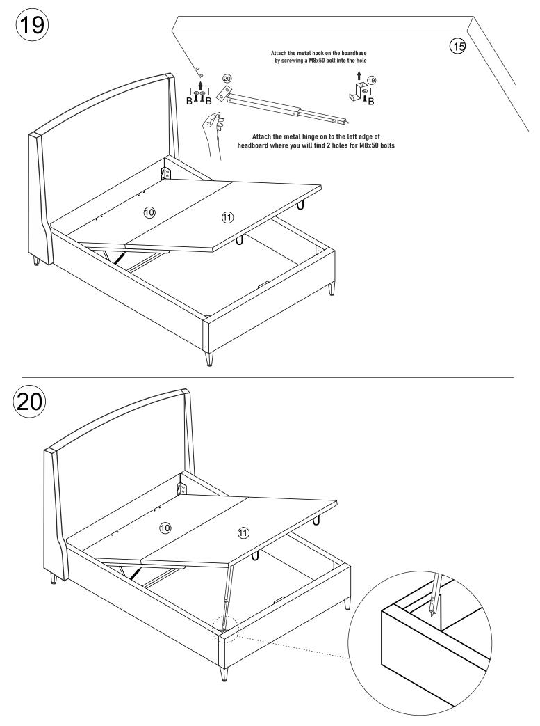
Fix the metal tube to the slot as in the picture.
